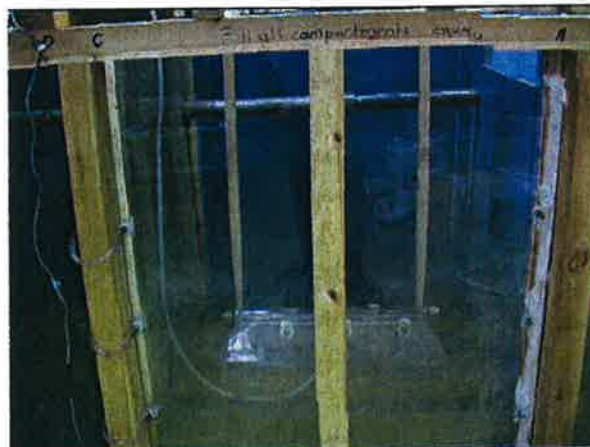
Figure 18 Sealed caisson compartment arrangement (Series 2)
