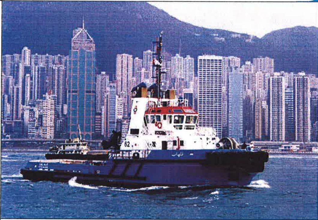
Stern tug, 2 x SRP 1515 CP (1850 kW each), 80 t bollard pull Shipyard: Cheoy Lee Shipyards Ltd, Hong Kong Owner: Wijnmuller Salvage BV, The Netherlands
