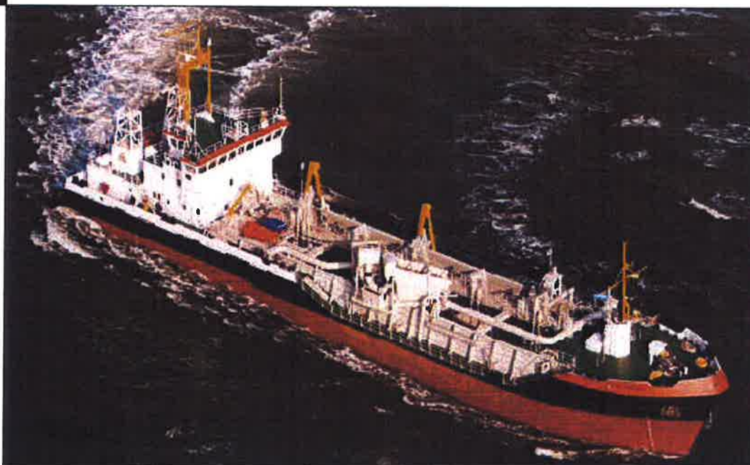
Suction hopper dredger, 2 x NAV 1010 (876 kW each) Shipyard: Scheepwerf Bijholt, The Netherlands Owner: Naßbaggerei Anton Müsing, Germany.
