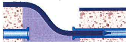
Figure 30. Typical Slip Lining Operation
