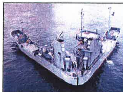
Pollution control and recovery vessel 2 x SRP 350 LS CP (800 kW each) Shipyard: C. Lühring, Germany Owner: German Navy
