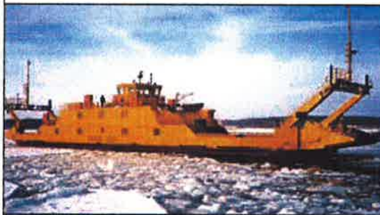
Double-ended ferry, 2 x SRP 350/350 (404 kW each) Shipyard: Åsi Verken, Sweden Owner: Swedish National Road Administration and Ferry Operation, Sweden
